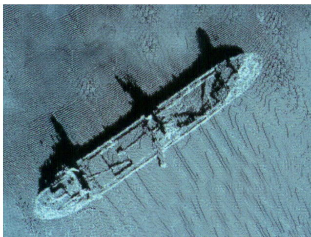
Fig.5 Sonar picture of ship's wreck founded on Persian Bay on the 50 m depth [3]
