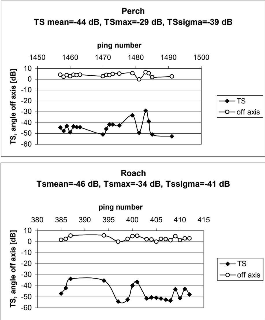
Fig. 1. An example of ping-to-ping variability of TS and degree off axis (in DB) for perch and roach during consequent fish passes through the beam
