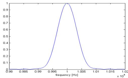
Fig. 4. Normalized amplitude spectrum of the Gaussian pulse shown in Fig. 2.
