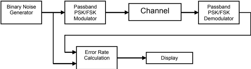
Fig. 8. Transmission simulator block diagram
