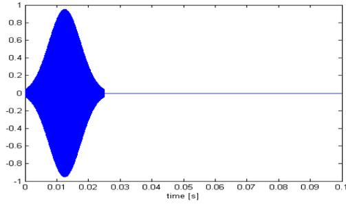
Fig. 2. Gaussian pulse, 10 kHz, 25 ms.
