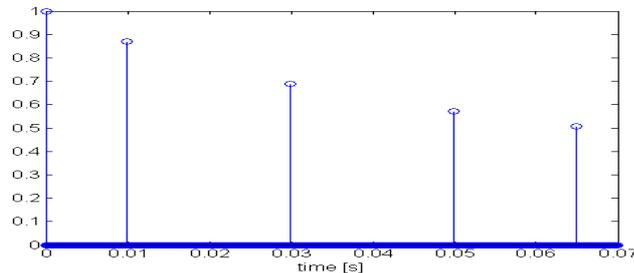
Fig. 1. Normalized impulse response of a channel with four reflections with delays:  $t_1 = 10ms$ ,  $t_2 = 30ms$ ,  $t_3 = 50ms$ ,  $t_4 = 65ms$ .
