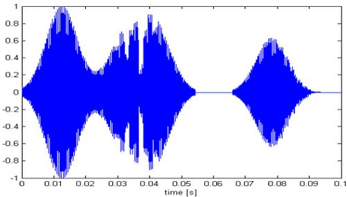
Fig. 6. Response of a nonstationary channel to the 25 ms, 10kHz Gaussian pulse. Channel parameters: 4 reflections, response duration 70 ms, sampling frequency 32kHz.
