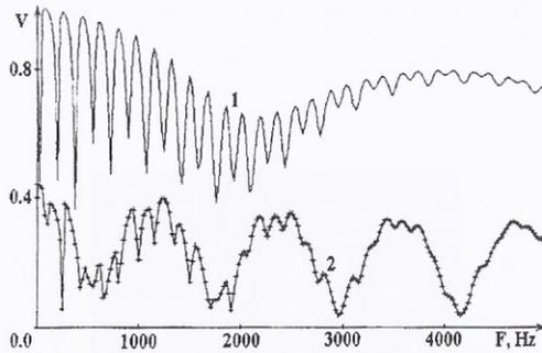
Fig. 4 Influence of absorption on resonance peaks
