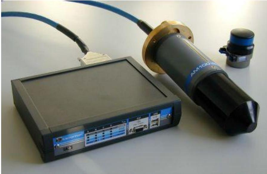
Fig.5. Underwater navigation system for the measuring module positioning.
