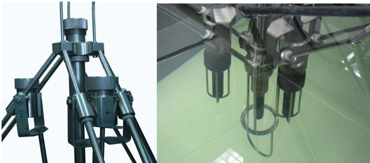
Fig. 1. The fragment of construction of multi-sensor array. On the left without hydrophones, on the right with hydrophones in water tank
