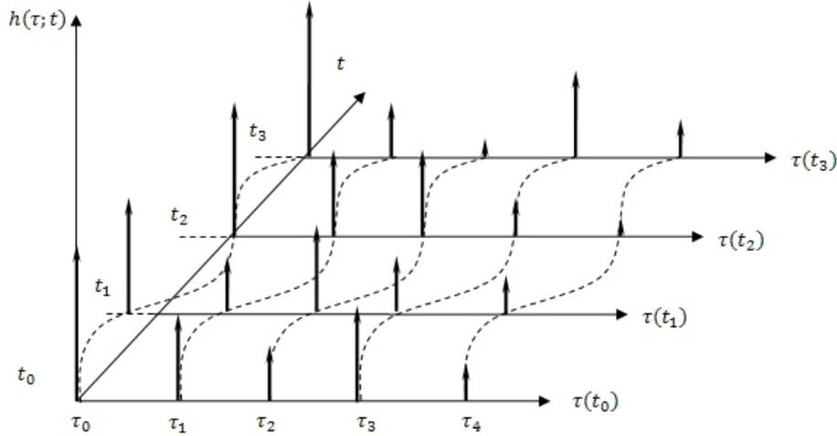
Fig. 1. An example of time-varying discrete-time impulse response
