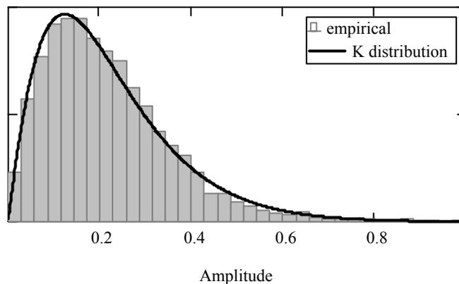
Fig.4a. The comparison of K distribution and empirical data histogram (nape of a neck)
