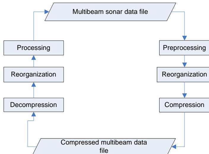
Fig.2 Overall diagram of multibeam data compression process
